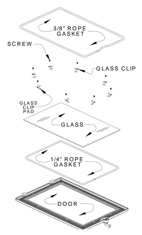
**Figure 1: Front Door Gaskets & Components**
