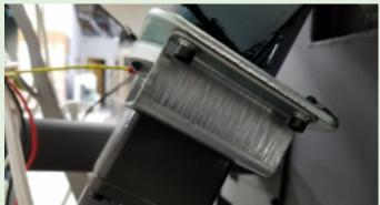
Remove all 4 of these bolts using a #4 metric allen wrench
