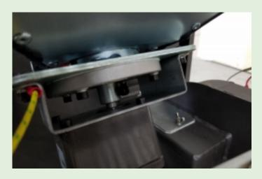
Once the set screw is loose, you will be able to drop the auger motor down from the bit assembly.
