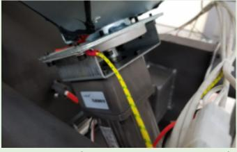
Once these are removed, you will need to loosen the set screw that holds the post of the motor to the bit itself. (This is the screw that is perpendicular to all the rest).  This set screw is removed with a #5 metric allen wrench \*Note that the Ubracket will only allow you to access the set screw from the front or the back)
