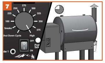
Before using your grill for the first time, it will need to be seasoned. Turn the temperature dial to HIGH and let run for 45 minutes with the door closed. After 45 minutes your grill will be seasoned. Turn the dial to SHUT DOWN CYCLE and allow the grill to run through its complete shut down cycle. Your grill is now ready to cook.
