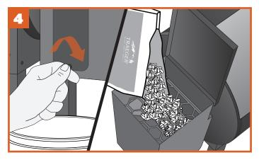
Once the hopper is empty, close the door, replace the fastener, and refill the hopper with a different flavor of TRAEGER® BRAND HARDWOOD PELLETS.
