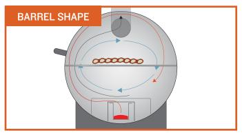
Traeger's signature barrel-shaped grill body creates a vortex of convection. It circulates hot, smoky air around the cooking chamber, surrounding your food with wood-fired heat for even cooking on all sides.
