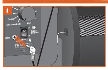
Insert the meat probe into the probe jack on the lower left corner of the controller, then thread probe through the access hole grommet on the left side of the grill body.
