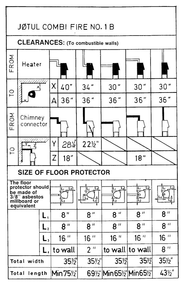
Fig. 1 Clearances and Floor Protector Size
