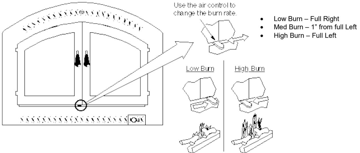
**Warning:** The air control becomes hot during operation - use gloves or a tool to prevent burns.
