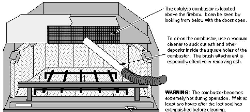
**WARNING:** The combustor becomes extremely hot during operation. Wait at least two hours after the last coal has extinguished before cleaning.
