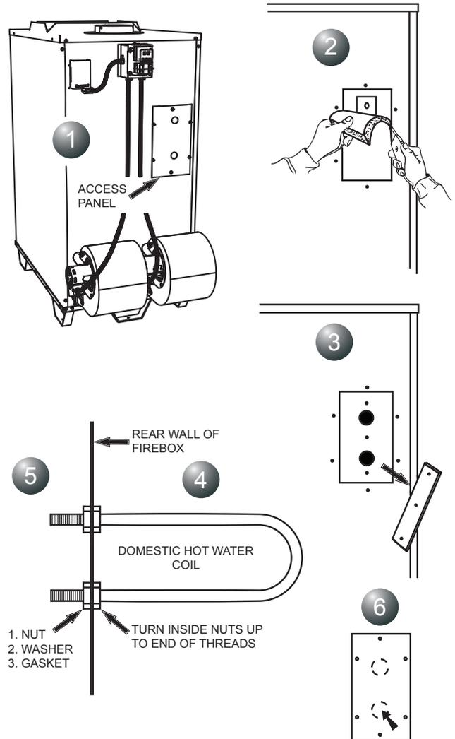
This Furnace will accept the installation of a Domestic Hot Water Coil Kit. The kit is a 1124 Water Coil and it may be purchased from your local dealer.
