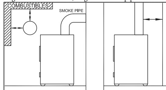
9" of combustibles provided an approved fire retardant material covered with 28 gauge sheet metal, spaced out 1" on non-combustible spacers, is utilized. See illustration.
