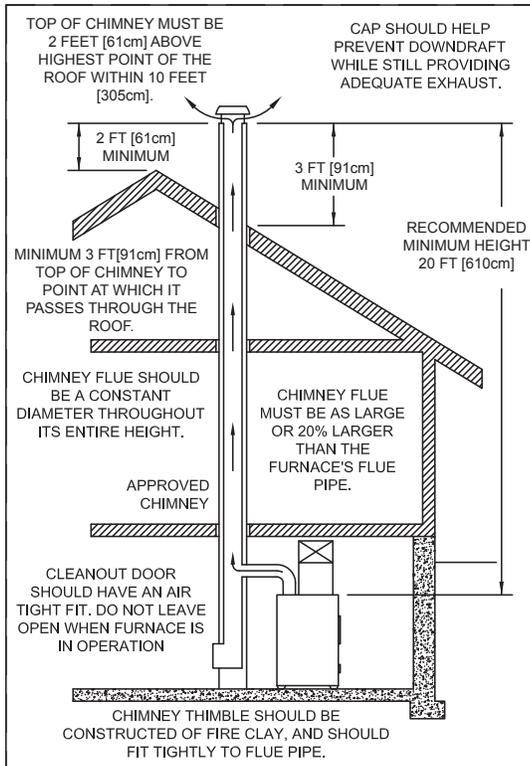
2. A masonry chimney should have a tile or stainless steel liner.
