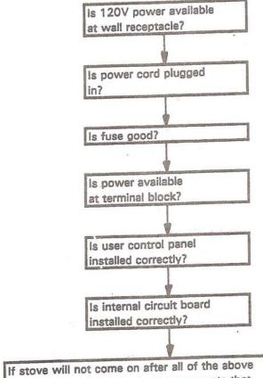
If stove will not come on after all of the above tests, then the only two components that could be at fault are the user control panel or the internal circuit board.
